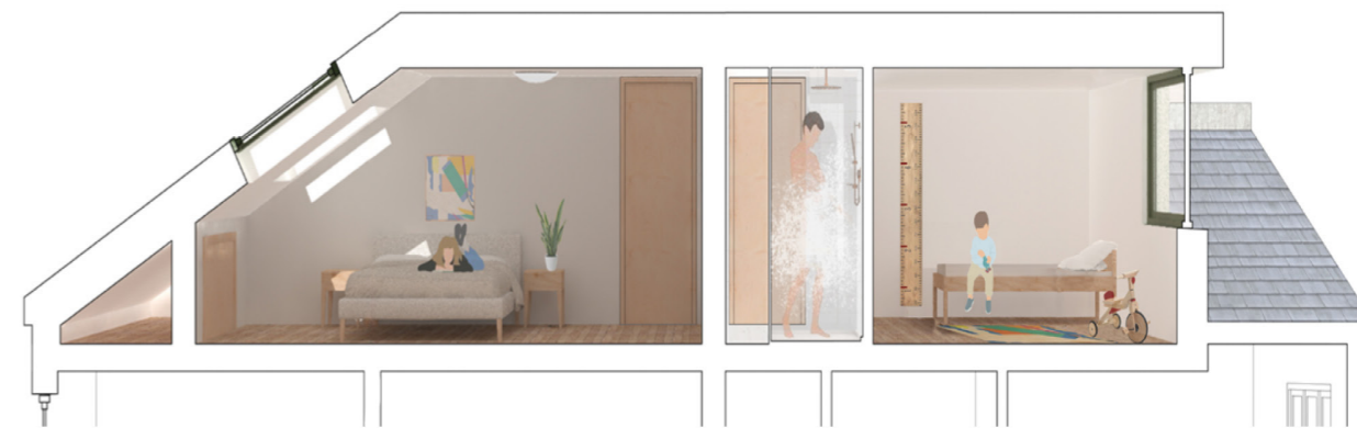
Permitted Development loft conversion resulting in lower ceiling heights and a smaller space due to rear step in.
