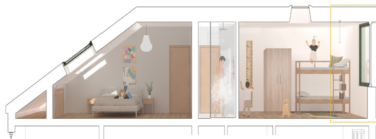
Great Green Lofts extension covering the whole house – creating two double bedrooms with full-height ceilings, with increased insulation to reduce heat loss.
